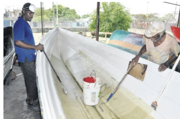
Phillip Berry, a boat maker at the Beechwood Avenue site in Kingston, uses an old boat to make the mould, an impression of the vessel. [Photo: Gleaner]
